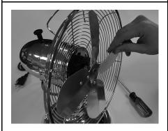
Slide the fan blade onto the mounting shaft with the shaft sleeve facing the motor. Align securing screw with flat groove in the motor shaft and tighten with Phillips screwdriver.
